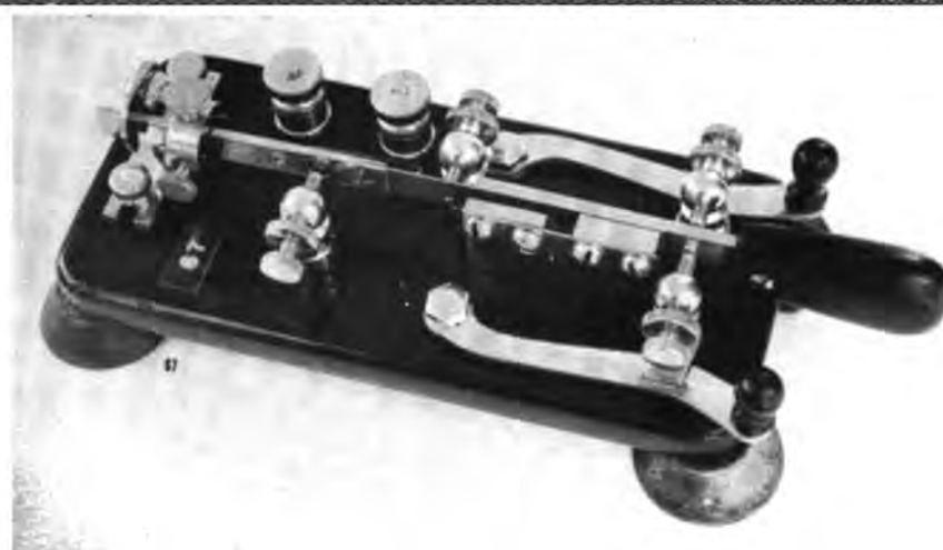
● (67) Signal Elec. Co. Semi-automatic key that can be converted to side-swiper by closing switches near paddle and locking down vibrator arm with clamp at far end of arm
